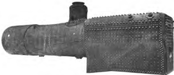
Fig. 148. Straight Top Boiler with Belpaire Firebox.
